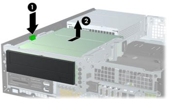
Figure 6-30 Removing the 5.25-inch Drive
